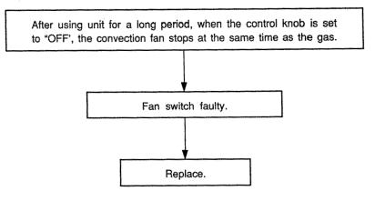
NOTE: After the main burner has lit, if the main switch is turned to 'OFF', in the period when the fan is operated by the 32 seconds delay timer (before the thermal switch closes), the fan will stop immediately.
