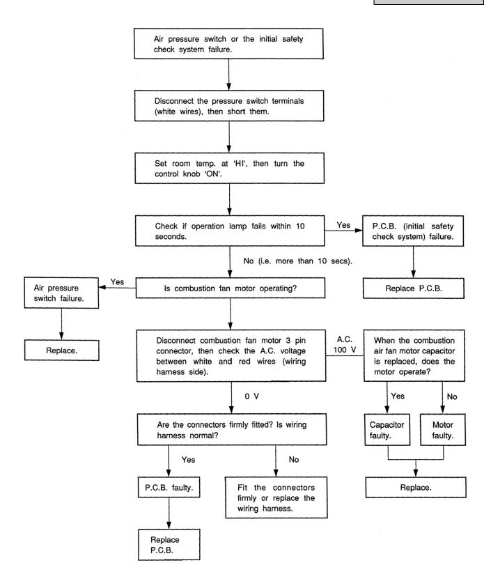
NOTE: When the ambient temperature is extremely low, it may take considerably longer for the air pressure switch to operate.
