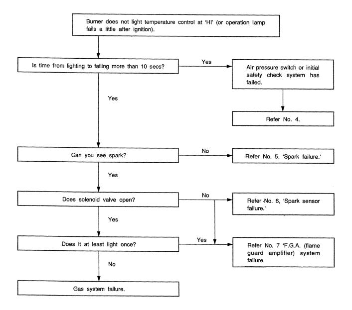
NOTE: Ignition sequence is repeated once again if the initial sequence fails to ignite burner.
